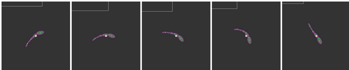
Figure 4.2: Generated motion sequence of a five-link swimmer turning. The swimmer turns by bending and undulating to create a smooth turn.
