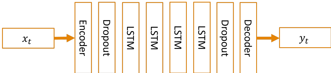
Figure 3.1: The network architecture used to model the direct distillation controller.
